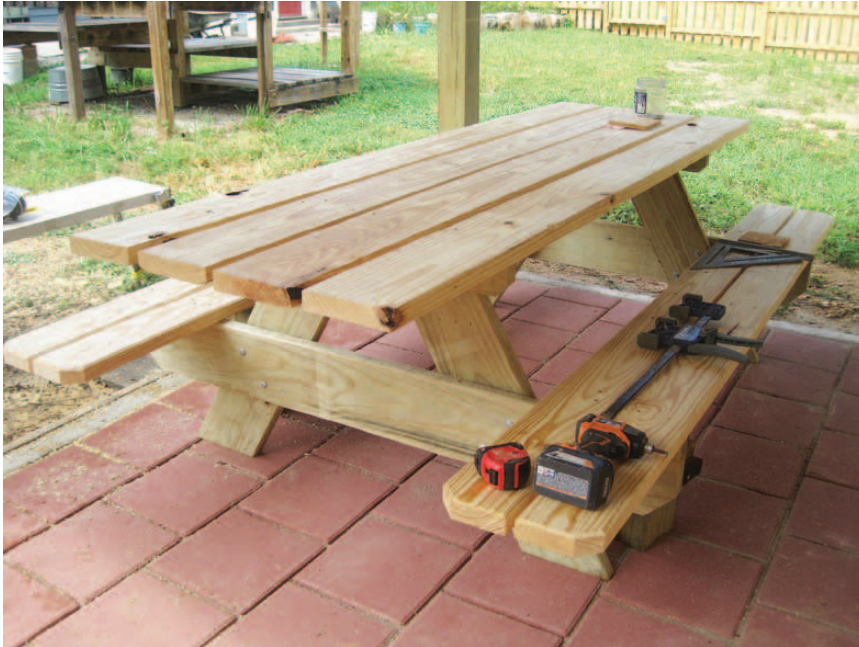
Attaching the top boards — the table top should measure exactly 31½ inches across if using a tile pattern that will measure 32 inches across.
