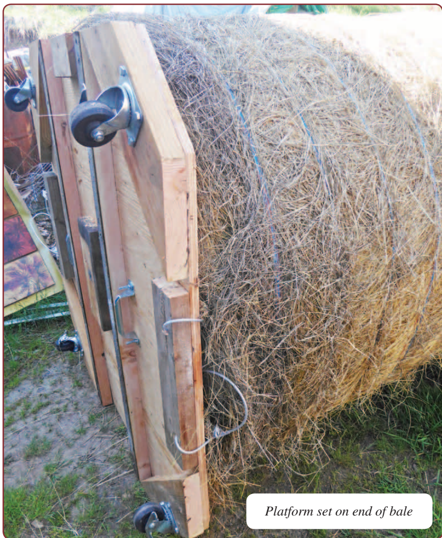
Figure 4: Angle iron supports and metal handles for lifting the cart to position it
