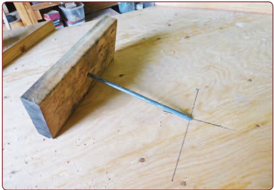
Figure 3: Spike creation and location of center hole
