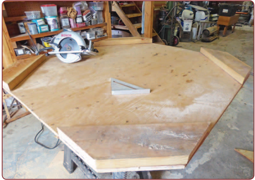
Figure 2: Attached 2x6 corner protectors/wheel bases
