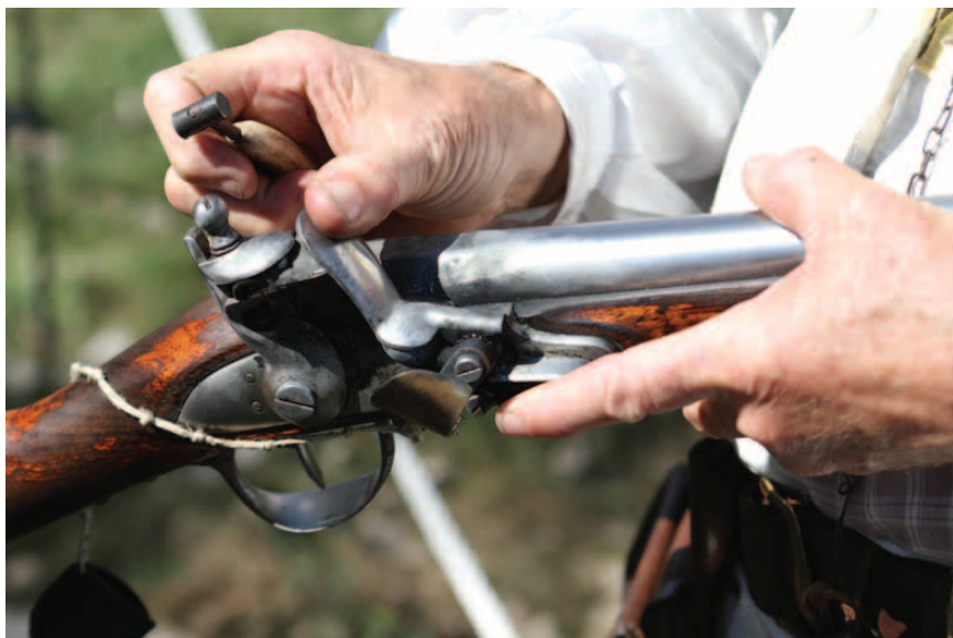
This flintlock is about to be “primed” with fine grain gunpowder.
