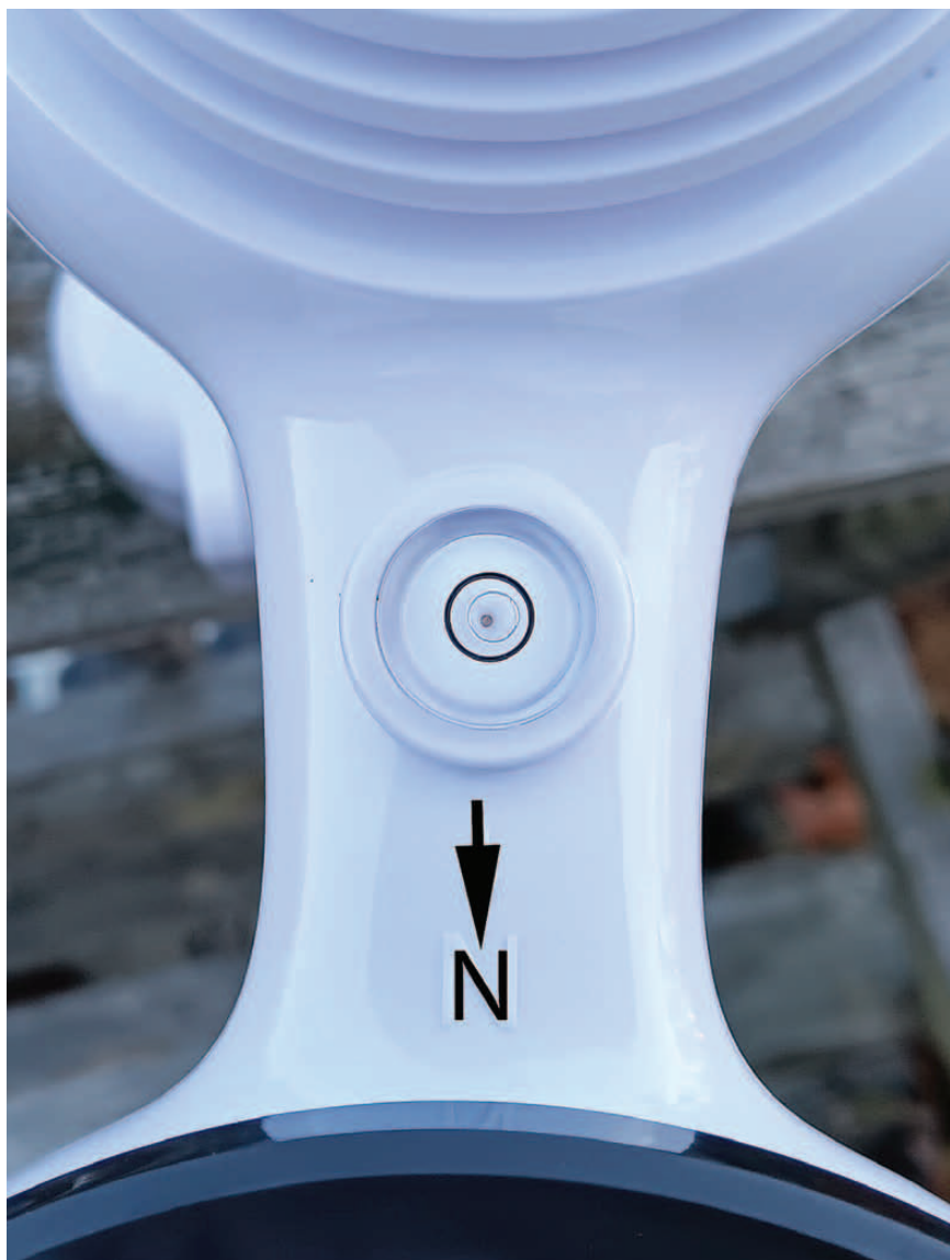
Bubble level built into one arm of the outdoor unit
