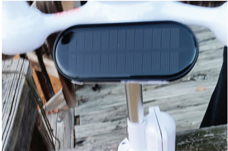
Some weather stations include a built-in solar panel to keep the internal battery fully charged.
